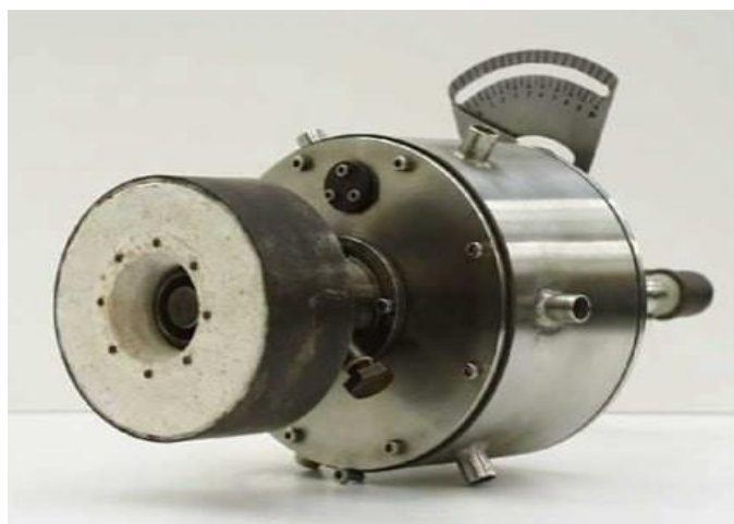
Fig 1. 30 kW IFRF research burner
